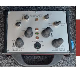
Turning wheels supporting the harvester's maneuvering, additionally equipped with the function of hydraulic lifting of the harvester on the wheel columns
